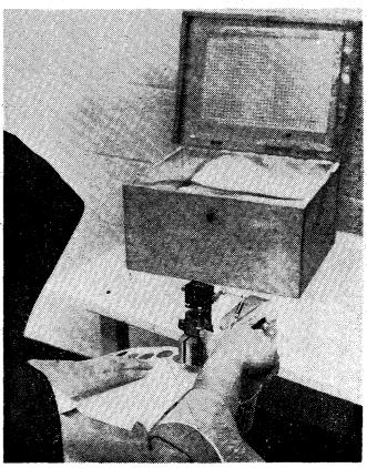
Electric Cutter Punches Small Hosts From Bread Sheet
